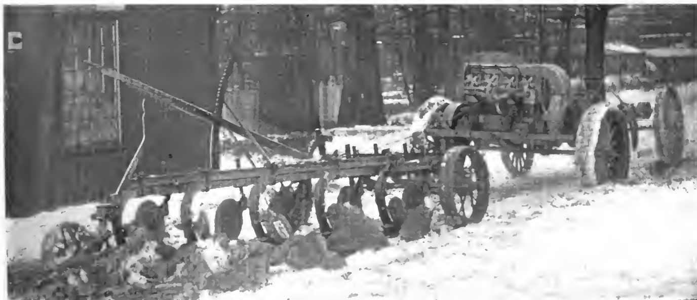
THE FRAYER-MILLER FARMOBILE PULLING FIVE PLOWS IN FROZEN GROUND NOT BROKEN PREVIOUSLY IN 25 YEARS
